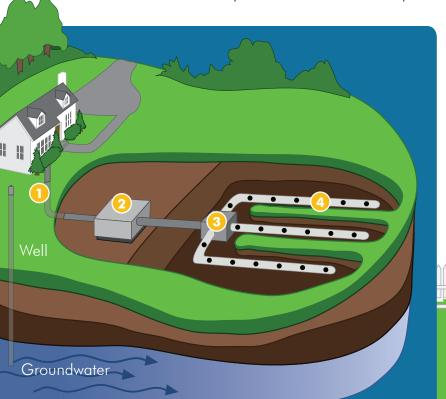
4. Once in the drainfield, the wastewater percolates into the soil, which reclaims the water for future reuse by naturally removing harmful bacteria, viruses, and some nutrients.
