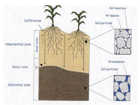
The size of the soil particle plays a crucial part in determining the amount of water it can hold and how fast the water passes through. Porosity is defined as the water-bearing capacity of soil particles that is due to both the number and size of pores and the extent to which they are interconnected. Clay has the highest porosity, when compared to sand or gravel, because it has many, very tiny pores which hold onto a lot of water.
